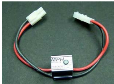
Chave de controle (Auto Discharge Cut Off Switch)
