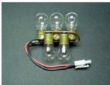
Medium Light Bulb Battery Discharger
